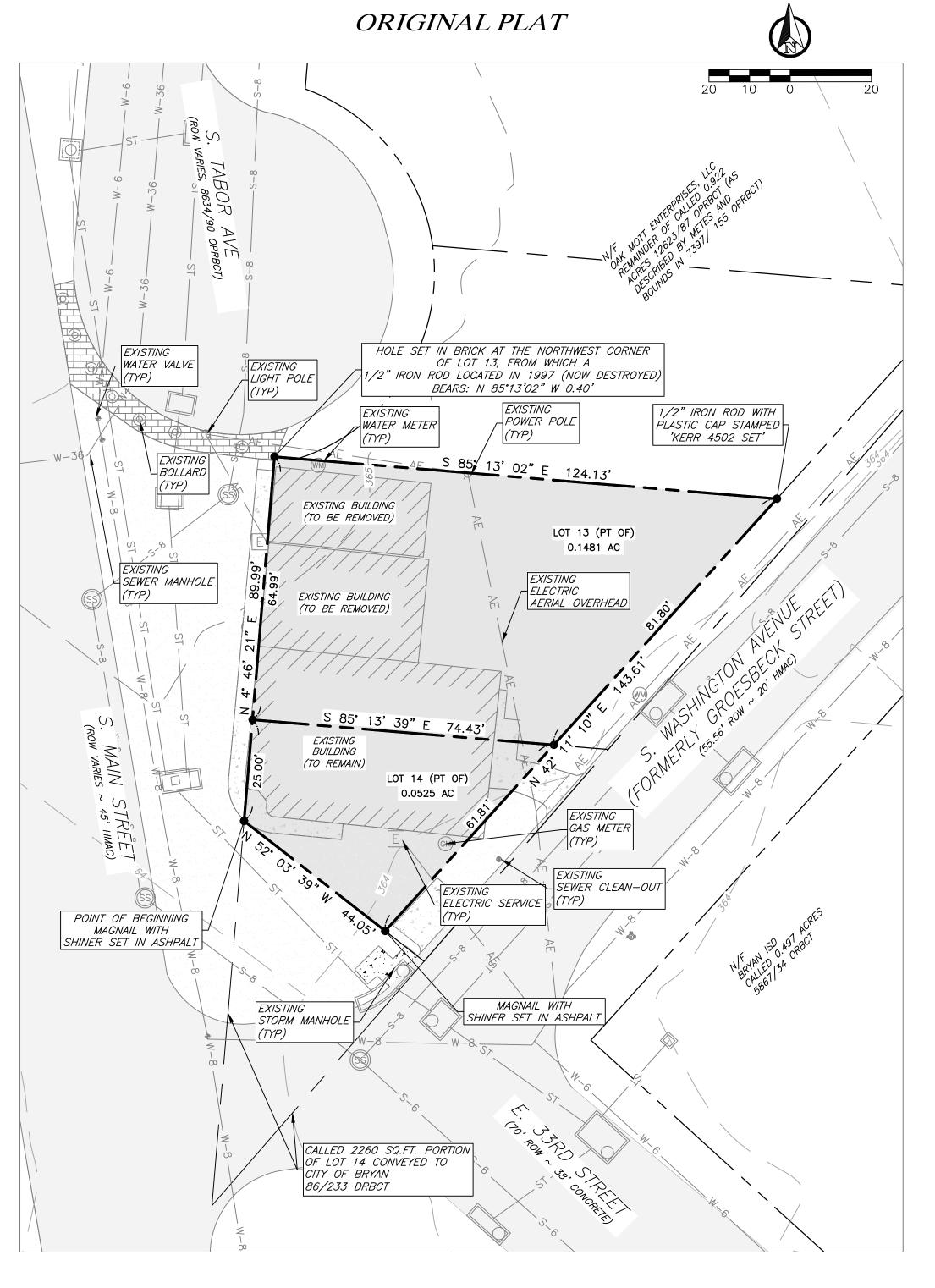
HOLE SET IN BRICK AT THE NORTHWEST CORNER OF LOT 13, FROM WHICH A 1/2" IRON ROD LOCATED IN 1997 (NOW DESTROYED) BEARS: N 85°13'02" W 0.40' 1/2" IRON ROD WITH PLASTIC CAP STAMPED 'KERR 4502 SET' S 85° 13′ 02″ E 124.13′ LOT 13R 0.2006 ACRES POINT OF BEGINNING MAGNAIL WITH SHINER SET IN ASHPALT MAGNAIL WITH SHINER SET IN ASHPALT CALLED 2260 SQ.FT. PORTION OF LOT 14 CONVEYED TO CITY OF BRYAN 86/233 DRBCT
